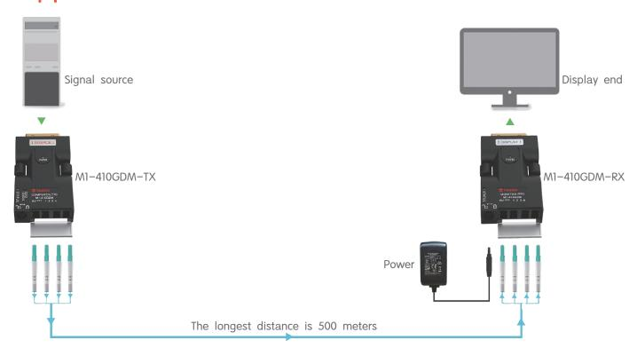
Four-core multi-mode OM3 optical fiber cable(LC)
