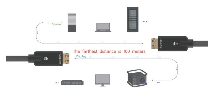
\* GDH03-xxMlt is a unidirectional active optical cable, so please determine the correct direction before deploying cable
