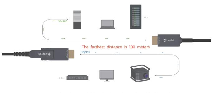
\* AHDxx-C is a unidirectional active optical cable, so please determine the correct direction before deploying cable (Connect the 'Source' end to the signal output device and the 'Display' end to the display device)
