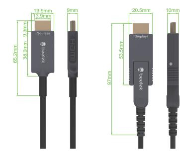
Connector Dimensions HDMI Type A Male: 65.2 \* 19.5 \* 9mm; Detachable connector: 47.5 \* 13.7 \* 10.2mm
