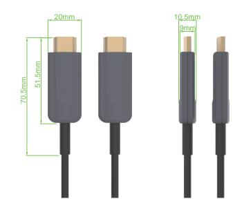
Connector Dimensions HDMI Type A Male: 70.5\*20\*10.5 mm
