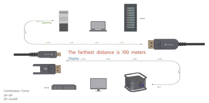
\*ADP8Kxx is a unidirectional active optical cable, so please determine the correct direction before deploying cable (Connect the 'Source' end to the signal output device and the 'Display' end to the display device)
